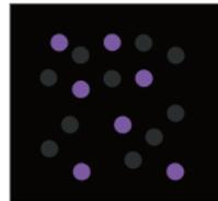
STEP 3 High intensity illumination results in fluorescence emission from the activated reporter dye.
