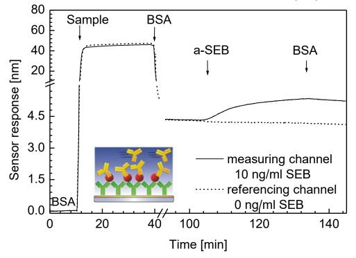
Example of reference – compensated measurement for suppressing of the effect of unspecific sorption and drift.
