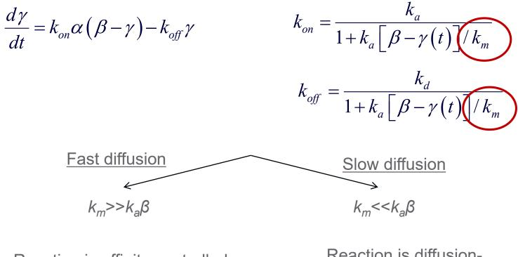
Reaction is affinity-controlled and  $k_{on} \approx k_a$ ,  $k_{off} \approx k_d$  Reaction is diffusioncontrolled,  $k_{on} \approx k_m \beta^{-1}$  and  $k_{off} \approx k_m k_d (k_a \beta)^{-1}$
