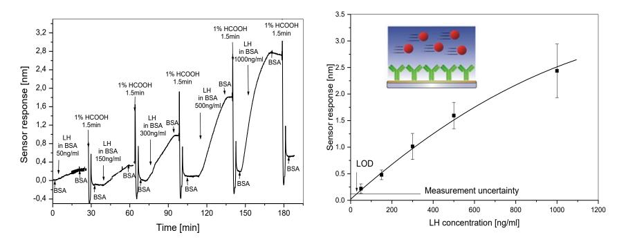
Binding kinetics for increasing concentrations of LH and regeneration between detection cycles (left) and the calibration curve (right).
