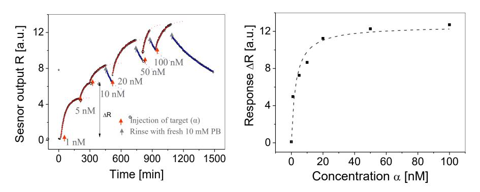
By fitting the dependence of equilibrium sensor response R on the analyte concentration  $\alpha$  the association affinity constant  $K_a$  can be fitted from a function:
