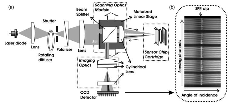
Example optical system for rapid scanning of SPR response over a 2D arrays of sensing spots with angular interrogation.
