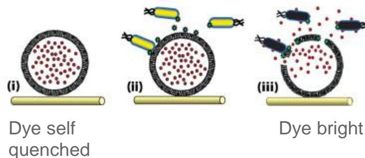
Fluorescent dye loaded to lipid vesicle, toxic bacteria destroy the lipid bilayer wall and leaches the dye reporter.
