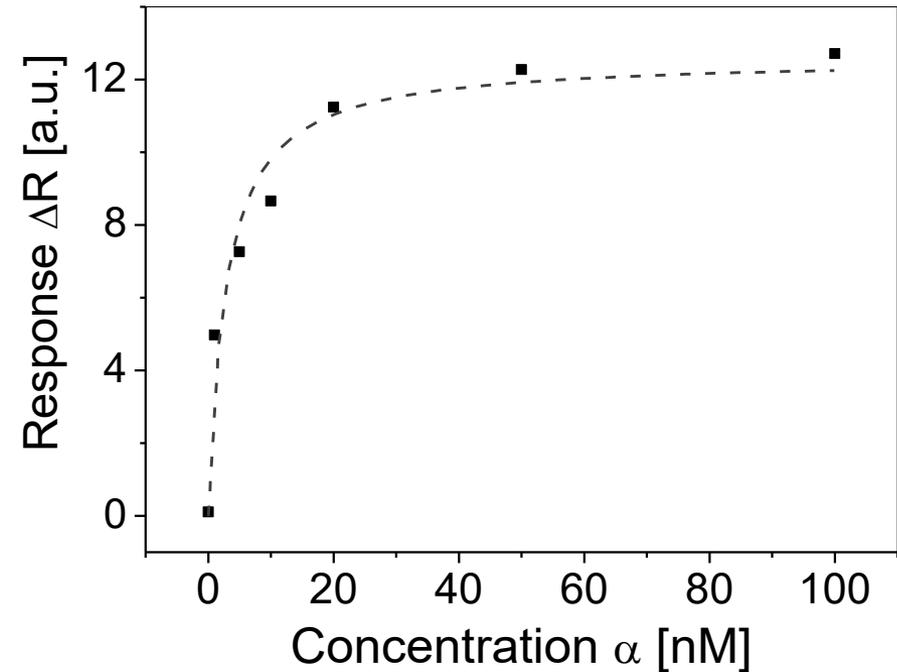
By fitting the dependence of equilibrium sensor response  $R$  on the analyte concentration  $\alpha$  the association affinity constant  $K_a$  can be fitted from a function:
