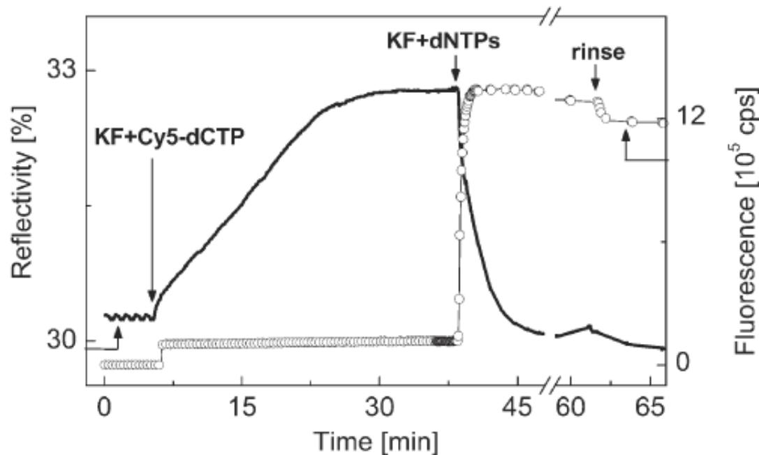
**SPR** - Mostly sensitive to binding of large KF to DNA probes.
