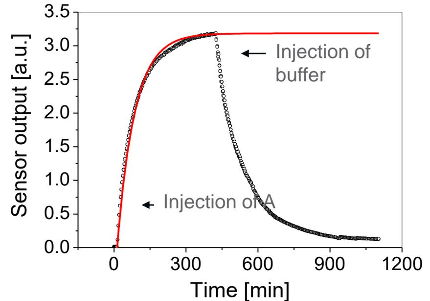
SPR biosensor output  $R(t)$  is proportional to  $\gamma(t)$ , one can fit  $k_a$  and  $k_d$  as:
