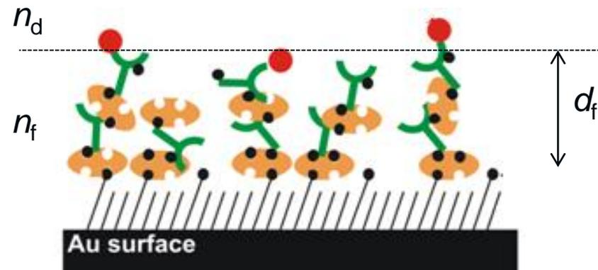
For most polymer materials holds  $\partial n_f / \partial c \sim 0.2 \text{ mm}^3 \text{ mg}^{-1}$  and in aqueous samples  $n_d = 1.33$ . For instance a full packed IgG monolayer exhibits  $\Gamma \sim 4 \text{ ng/mm}^2$ , IgG hydrodynamic radius  $R_h \sim 5 \text{ nm}$ .
