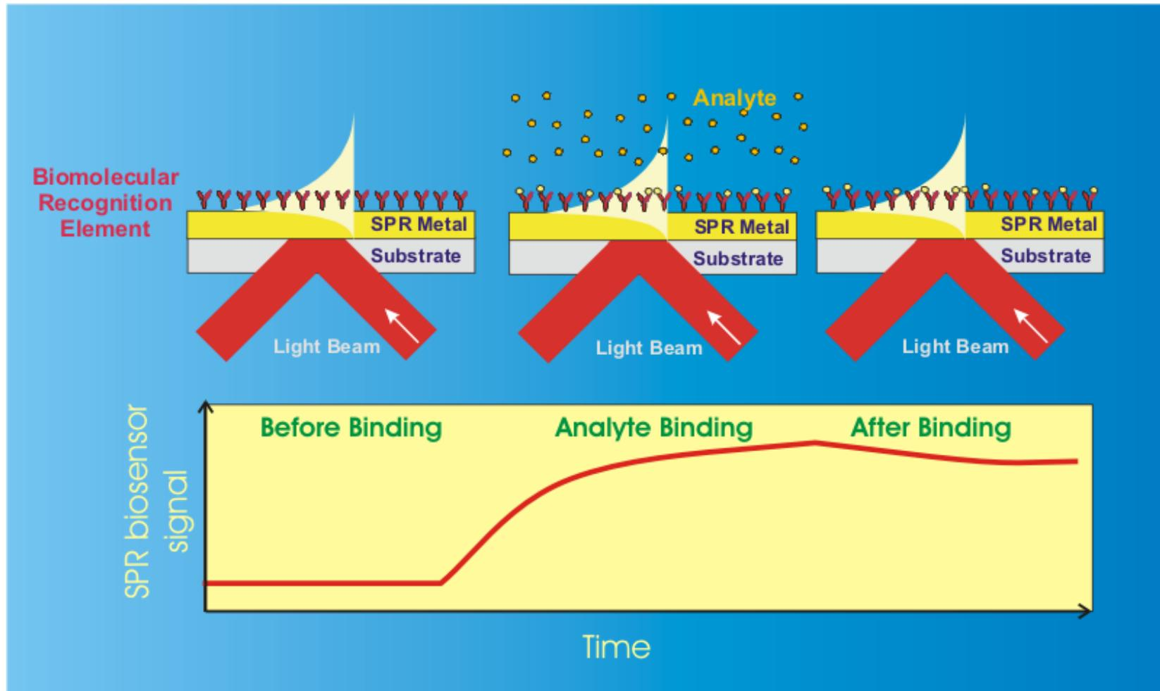
SPR signal = LSPR wavelength  $\lambda_{LSPR}$ , SPR coupling angle, or wavelength
