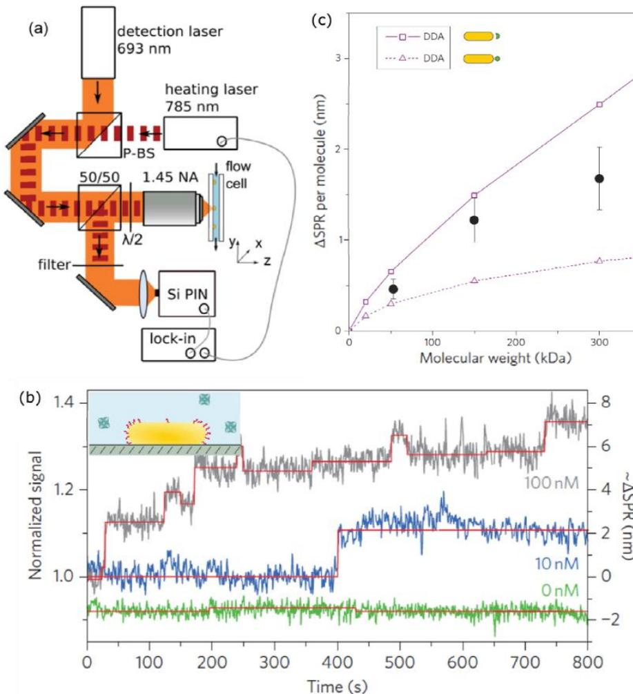
Tracking LSPR wavelength allows for monitoring of individual on and off binding events.
